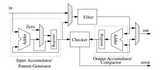
Figure 1. On-line/off-line BIST hardware
