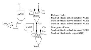
Figure 4. A typical full-adder implementation
